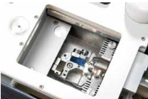
Rotate the knife holder into „trimming position“.
