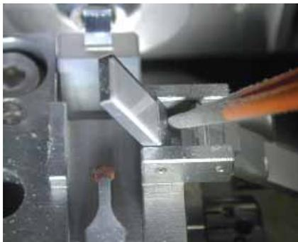
Pull back grid holder towards you and flip bridge to the right using a pair of forceps.
