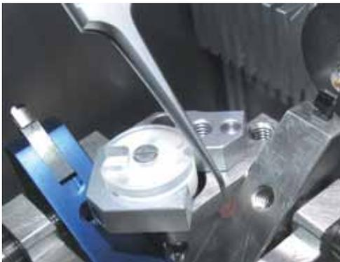
If you want to place the grid in the grid-box move the grid-box holder aside with tweezers and retract the forceps holding the grid.
