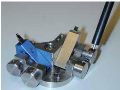
Lock the knife by turning the locking screw clockwise.
