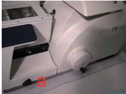
Lock the FC7 cryochamber to the chassis of the Ultracut UC7 by turning the lever „a“ clockwise until its end stop position.
