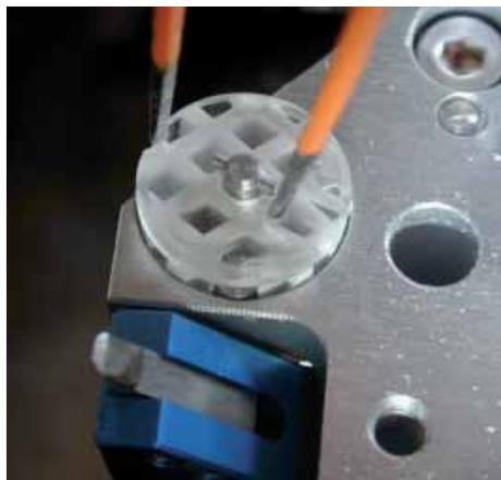
The transfer container can be removed using a pair of forceps.
