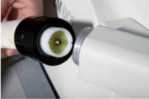
Connect the LN<sub>2</sub> hose with its threaded connection to the FC7 cryochamber.
