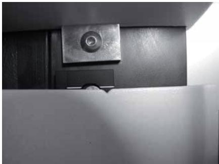
Slide on the chassis of the Ultracut UC7 until the second indentation line. Turn the hand wheel of the Ultracut UC7 to move the specimen arm to the lowest position.
