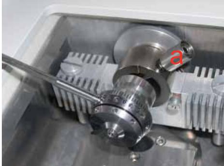
Insert the cryo specimen holder into the specimen arm.
