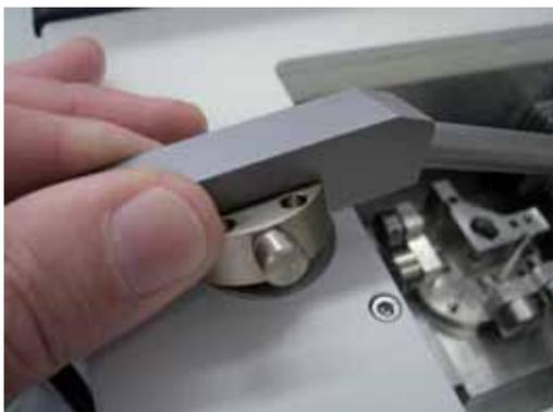
Place the antistatic electrode with its holder into its position on the cryochamber.
