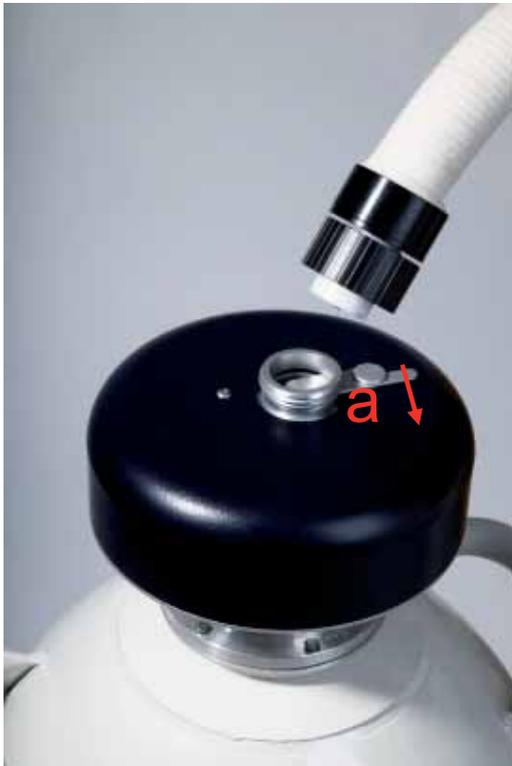
Connect the LN<sub>2</sub> hose with its threaded connection to the FC7 to the pump. Before inserting the connection open the safety shutter (a).
