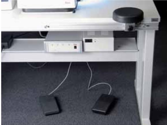
In case a Leica EM UC7 instrument table is available place the power supply onto the shelf beneath the table board.
