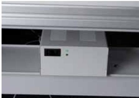
In case a Leica EM UC7 instrument table is available place the power supply onto the shelf beneath the table board. Connect the power supply to the mains.
