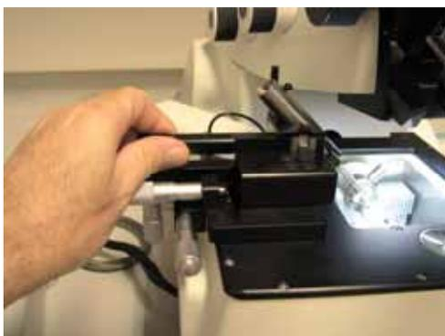
Lift up the forceps either by using the micrometer gauges or manually by gripping the z-direction lever.
