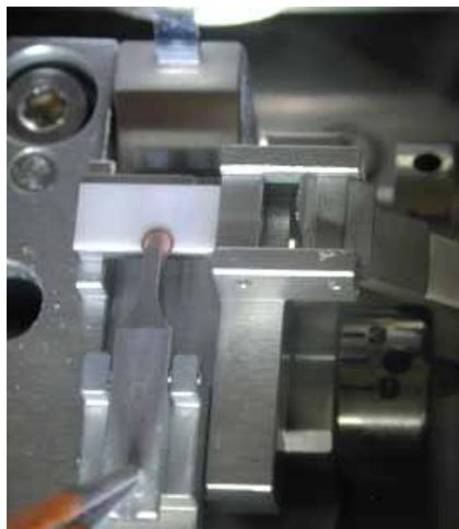
Open grid holder by pushing on the small indentation at the rear end with a small black lever or a pair of forceps. Move grid holder towards the grid and clamp it by releasing the clamping jaw.
