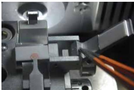
Close section press by using a pre-cooled pair of forceps.
