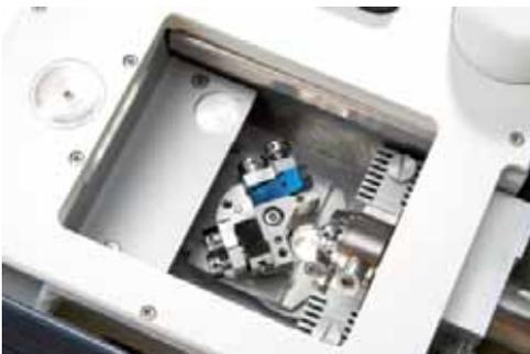
The rotating knife holder is now in the "loading position". It can only be inserted in this position.
