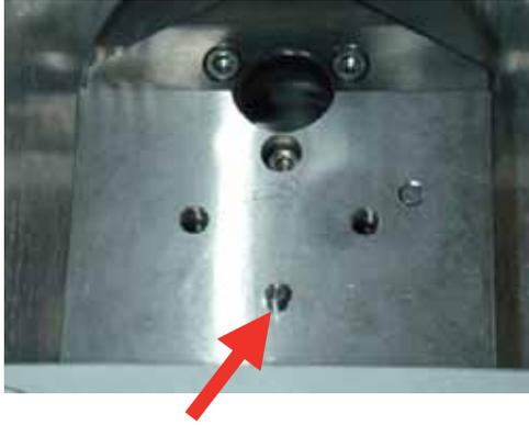
The knife plate in the cryochamber carries a pin (red arrow) that corresponds to the hole in the knife holder (red arrow).
