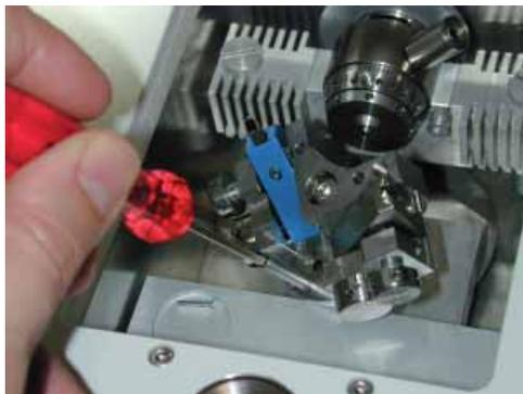
Insert the rotating knife holder containing knives into the chamber.
