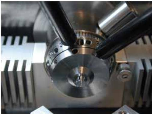
Lock the specimen pin in the cryo specimen holder.
