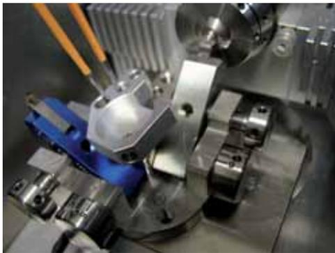
Place the grid-box holder with its magnet onto the knife holder.
