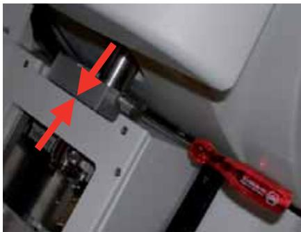
Guide the cryo specimen arm into the specimen arm of the Ultracut UC7. Slide the FC7 cryochamber into the chassis until you reach the end stop.
