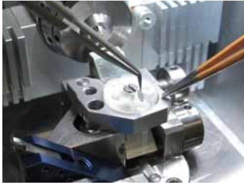
Adjust the grid-box using a pair of tweezers and the grid with the y and x movement of the manipulator in order to position the grid above an empty recess of the grid-box.
