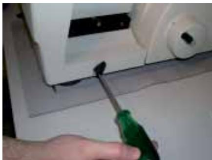
To increase the clamping remove lever „a“ by unscrewing slot screw. Reposition the lever an eighth counter clockwise on the clamping shaft and lock FC7. Repeat procedure until FC7 cannot be removed by gently pulling in south direction.
