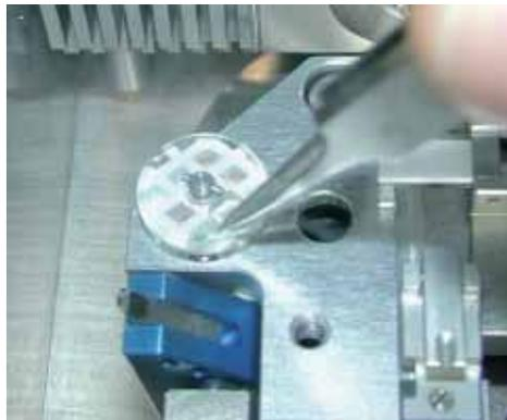
Transfer flattened grid into the transfer container.
