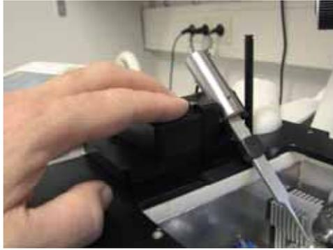
To prevent possible influence of the grid on the ionizer retract the forceps by pulling back the assembly.
