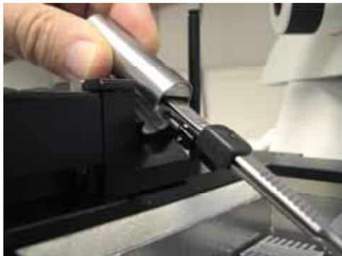
Insert the forceps in its holder of the micromanipulator and slide it towards the end stop position.
