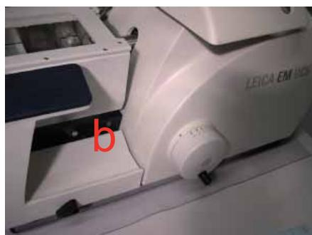
Push the knife plate of the EM FC7 until its north end stop position. Lock the knife plate to the knife stage of the Ultracut UC7 or UC6 by turning the lever b clockwise.
